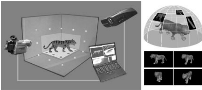
Figure 1: System overview: The stand over which is lying the 3D object to reconstruct is color marked for precise and automatic pose estimation. The calibrated projector adaptively projects color points over the measured room corner in order to automatically calibrate the video camera image. Each processed image from the live video camera is stored in a hemispherical distribution of views (top right) or in a most-recent image buffer list (bottom right) to ensure a balanced set of images for space carving. The current set of color voxels are interactively displayed for immediate reconstruction feedback from the latest set of images.
