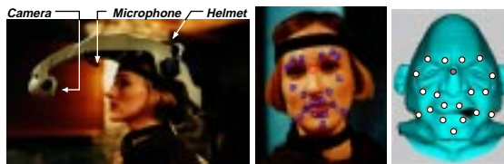
Figure 4. The tracking system
