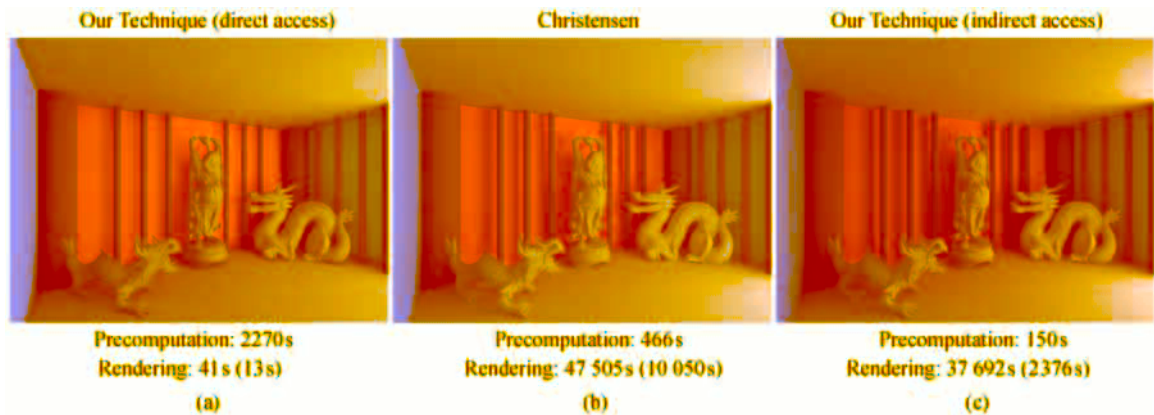
Fig.4. Scene with mostly indirect illumination. (a) Our technique using directly a 30 \times 20 \times 92 uncompressed grid (11.4 MB) constructed with 80 M photons. (b) Christensen's method reference image with 3200 rays to sample the hemisphere and 5 M photons stored (124 MB). (c) Our technique using indirectly a 12 \times 8 \times 20 uncompressed grid (590 KB) with the same number of photons shot and the same number of rays to sample the hemisphere.
